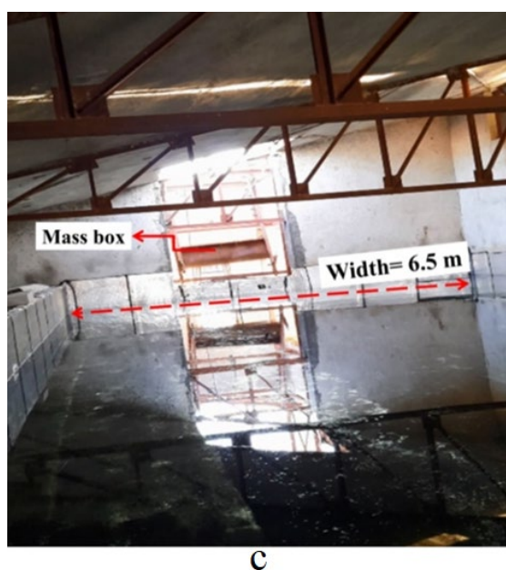
Fig. 1 a) A schematic front view of the laboratory-scale dam reservoir setup, b) A schematic top view of the laboratory-scale dam reservoir setup with two arrays spaced 76 centimeters apart, c) View of the laboratory-scale dam reservoir setup
