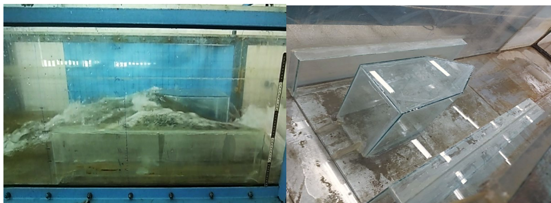
Fig. 2 Overview of the experimental setup and flow pattern visualization in a rectangular compound channel with a central baffle
