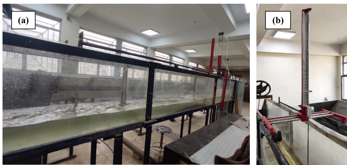
Fig. 1 View of (a) the experimental channel and (b) the depth gauge used in this study.
