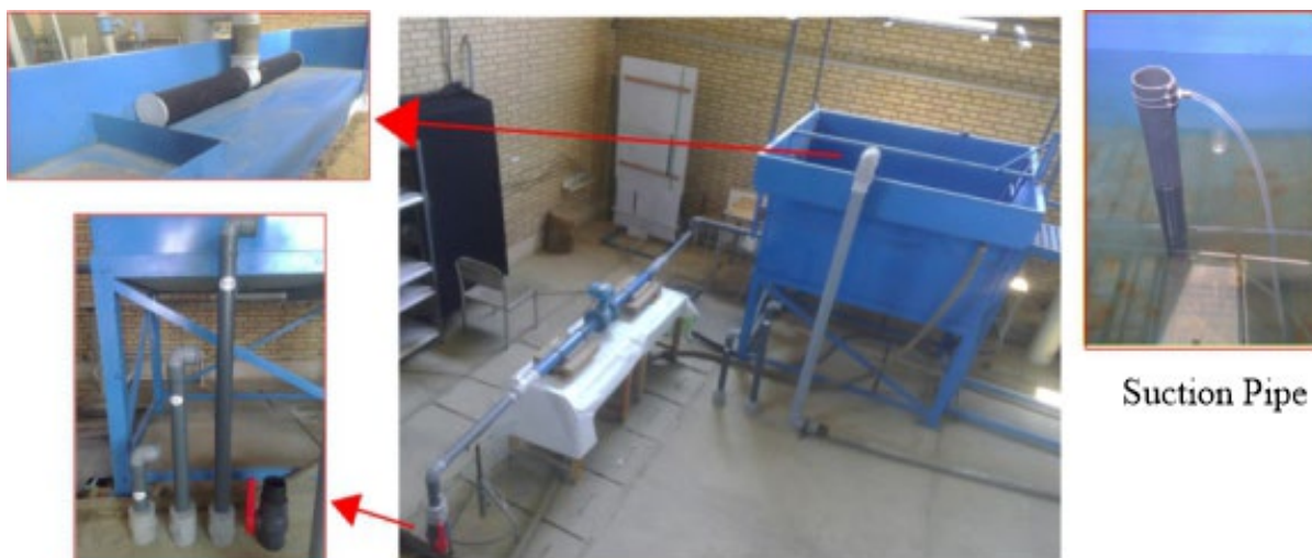
Fig. 2 The experimental setup including of reservoir, suction pipeline, head setting pipes and the flow inlet pipe
