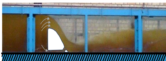
Fig. 2 Physical model of a crest Ogee spillway combined with a culvert at the bed level.
