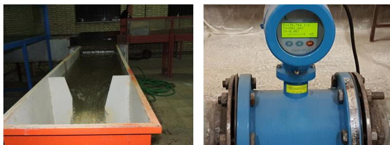
Fig. 6 Flowmeter (Megap 3000) and cipolletti Weir
