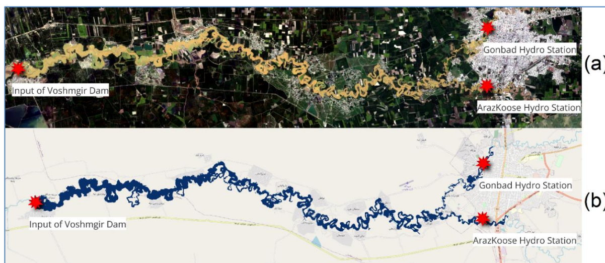
Fig. 5 Flood extent observed and registered by Sentinel-2 satellite (a) Sentinel 2 satellite RGB image (b) Detected flood extent from Sentinel 2 image
