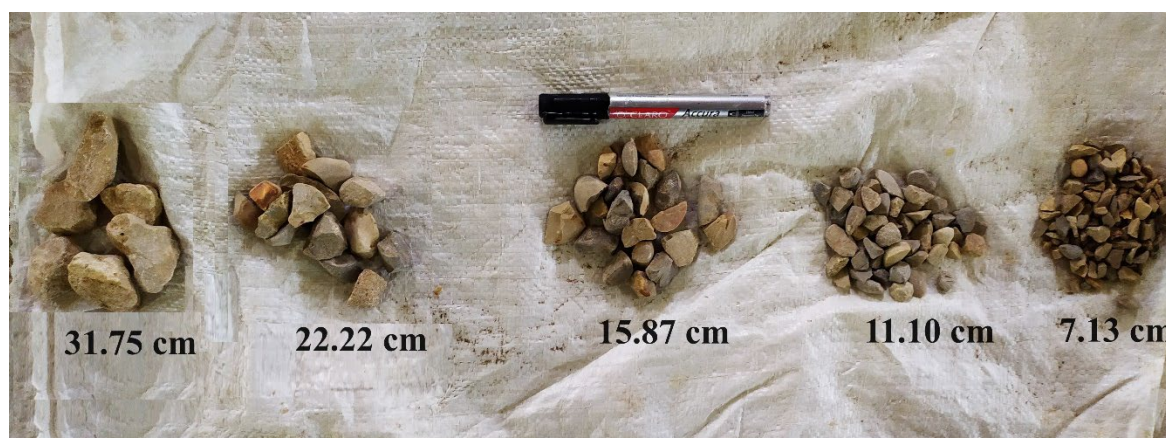
Fig. 4. Materials utilized for constructing porous weirs
