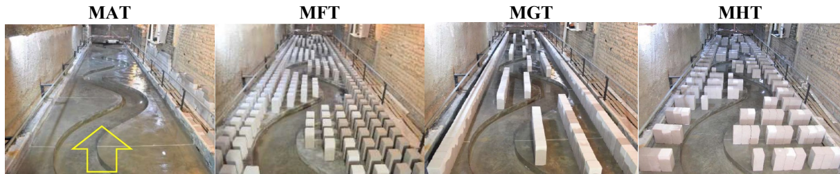
Fig. 1. The laboratory compound meandering channel with different building arrangements (Naghavi et al. 2023b).
