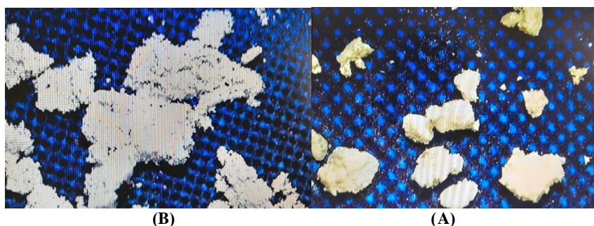
Fig. 1 Microscopic image from sample of Granite and Marble stone powder the scale: A) Marble, B) Granite
