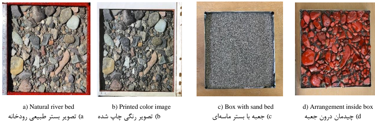
Fig. 6 The steps of arranging sediments inside the galvanized box
