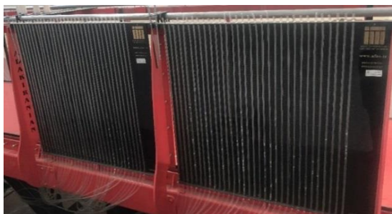
Fig. 5 Scaled board for piezometric height reading in the bottom and body of the laboratory flume
