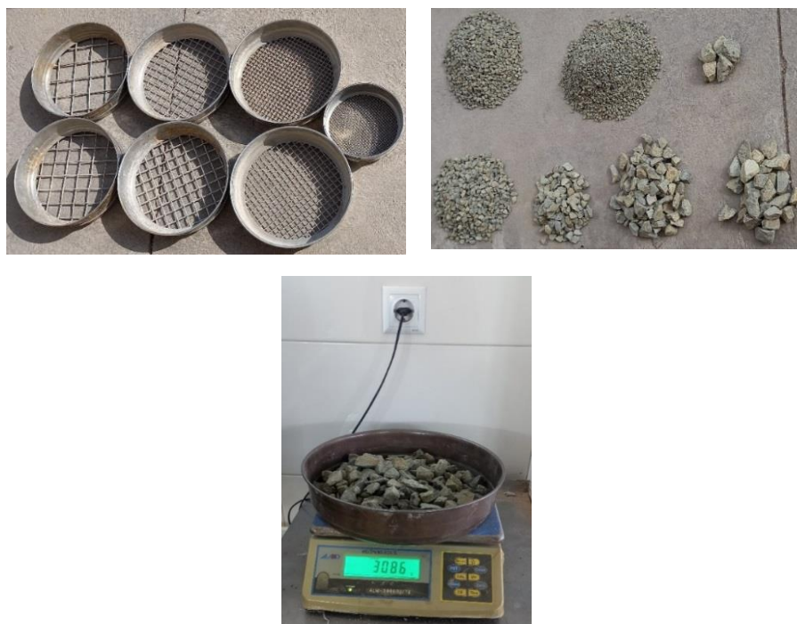
Fig. 3 The stages of granulation of rockfill materials in the quality control laboratory of Omran Beton Zanzan Company
