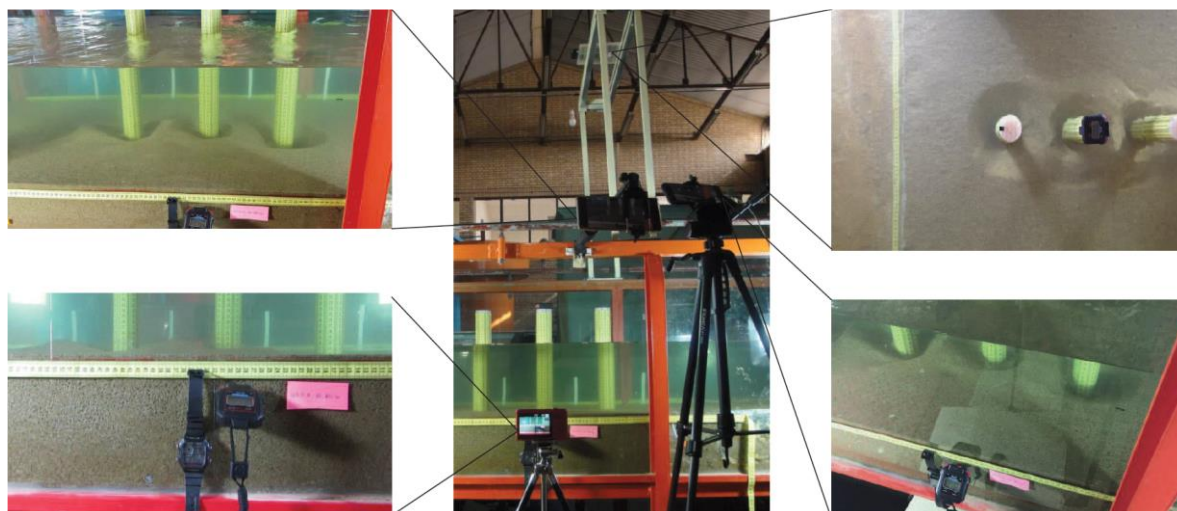
Fig. 3 Location of the cameras and the scouring process from their perspective
