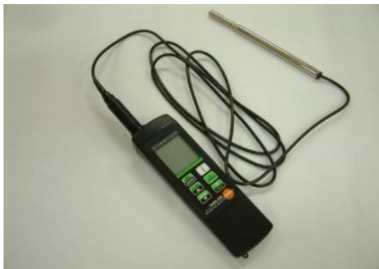
Fig. 3 velocity meter (Hot Wire) used to measure air speed
