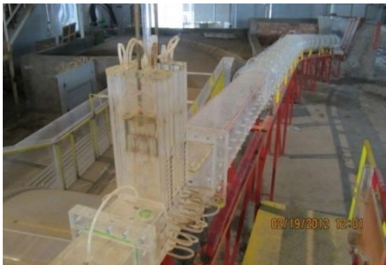
Fig. 2 View of the water transfer flume simulated with the lower drain of the dams
