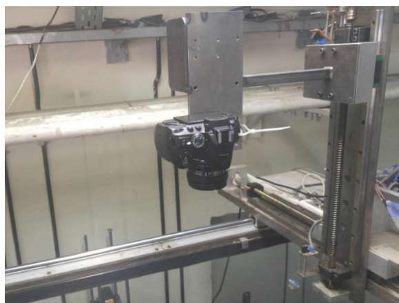
Fig. 3 Using camera for capturing of bed particle motions in the plan view
