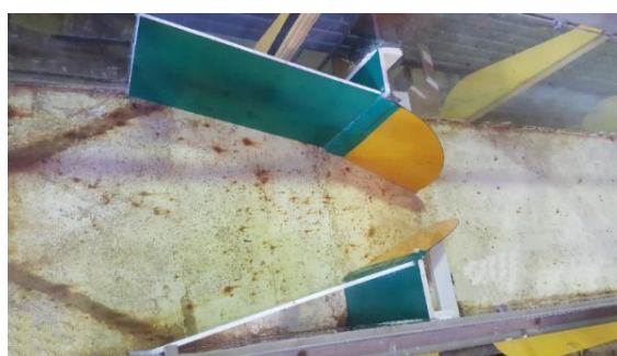
Fig. 4 Gradual conversion installed in the flume
