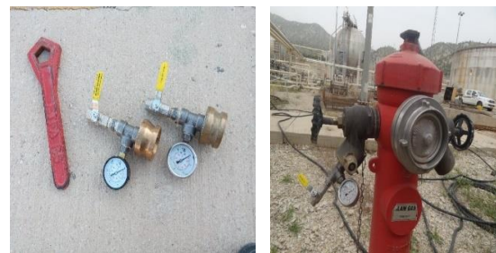
Fig. 3 Instruments and methods for measuring static pressure
