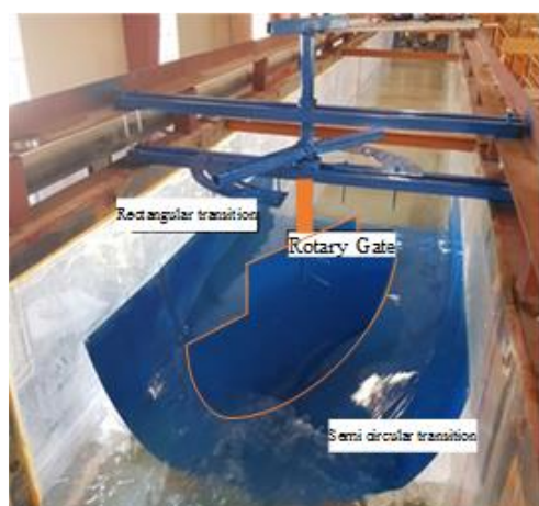
Fig. 2 The rectangular channel used in this research and the region of gate installation and transition in it
