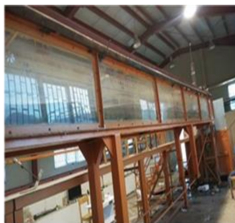
Fig. 2 The rectangular channel used in this research and the region of gate installation and transition in it
