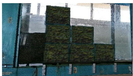
Fig. 2 Experimental porous stepped spillway
