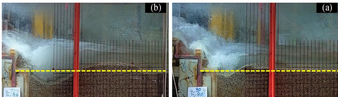
Fig. 8 A View of sediment ridge at the downstream of weir SL_2 : a) y_c/h=0.34 , q=0.02m^3/m.s and \eta=0.098 and b) y_c/h=0.61 , q=0.046m^3/m.s and \eta=0.52
