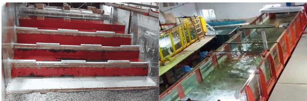
Fig. 3 Photos of experimental flume and stepped weirs
