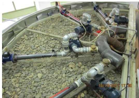
C- Placing parallel pumps on the model
