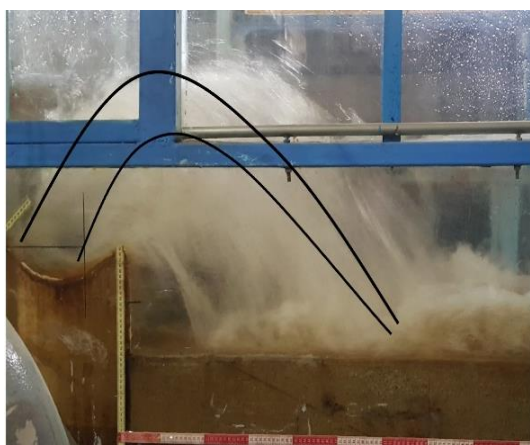
Fig. 10 A view of two jets created by deflectors.
