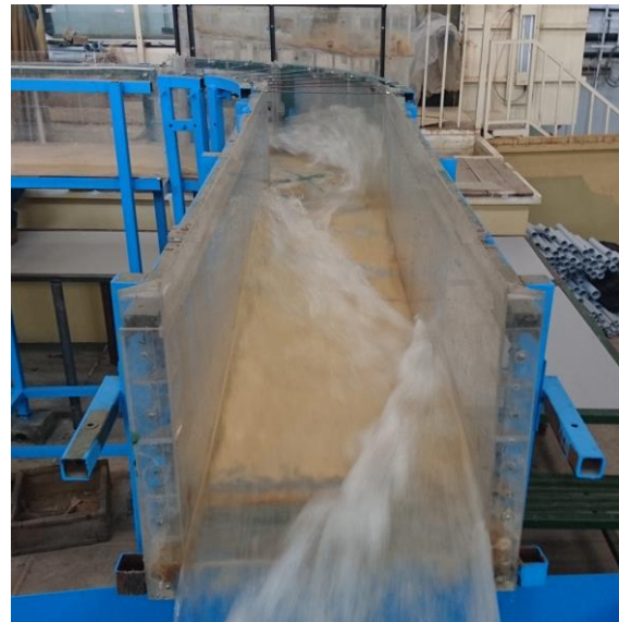
Fig. 12 Cross waves formation in the experimental flume and 3D model
