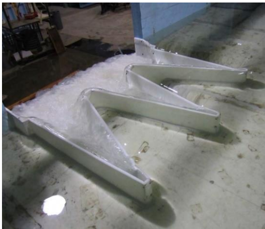
b) Laboratory model of Millsite Dam
