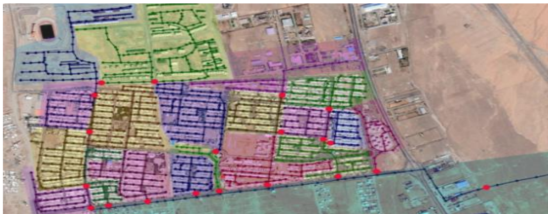
Fig. 2 Zoning of sewage network of Valiasr town (red circles indicate selected pipes in each area)
