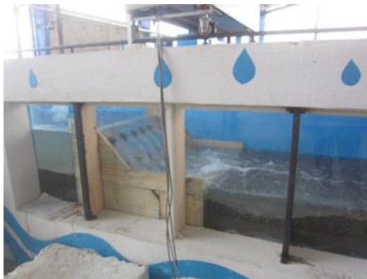
Fig. 7 Installed model in channel
