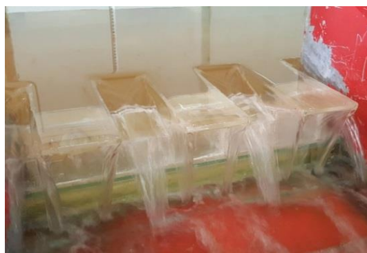
Fig. 7 A view of the Piano Key Side Weir P=15cm
