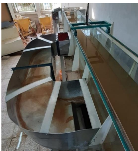
Fig. 9 A Plan View of the 10 m flume and the side channel
