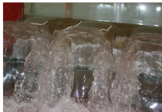
Fig. 8 A view of the Piano Key Side Weir P=20cm
