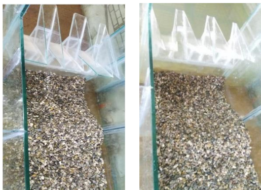
Fig 7 Scour profile in the downstream of the rectangular and trapezoidal PKW models
